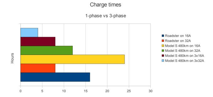
The data on this chart is based on 230V with no losses during charging. All the energy drawn from the grid goes into the battery with a 100% efficiency. For the Roadster I've used 53kWh for the battery capacity, for the Model S, 85kWh. In practice, it will result in even longer charging times than displayed.
