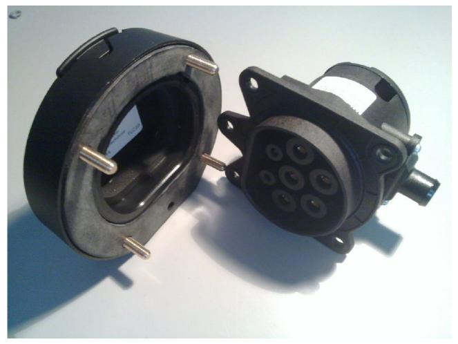
This is the Type 2 socket as I purchased it. There is also a interlocking actuator on top of the socket which isn't in this picture.
