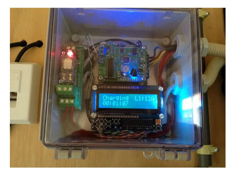
This is what it shows when an EV is charging! On this picture the EVSE was running a firmware where I limited it to 12A just for testing purposes.
